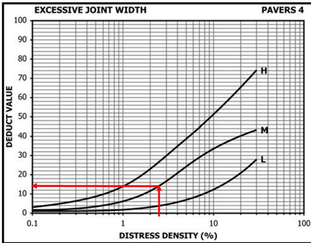
Figure 3-12 Excessive Joint Width Distress Deduct Curve
