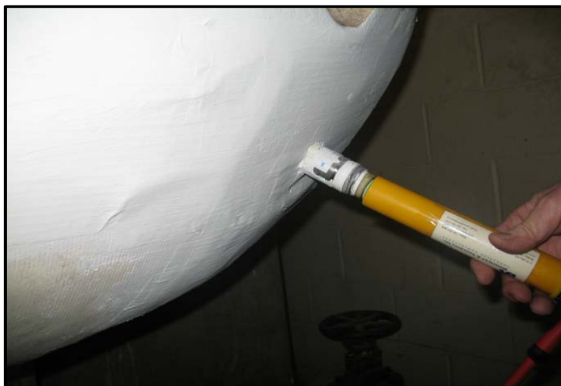
Figure B-37 Reference Electrode Placed in Contact with Moist Wadding Temporarily Placed Inside of the Capillary Tube Monitoring Port.
