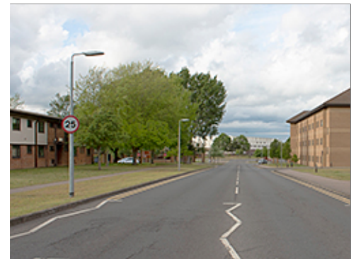
Detached Sidewalk with Landscaping
